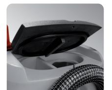
The easy access to the recovery tank allows fast cleaning and sanification of the tank; the tilting tank together with a large size drain hose allow the complete emptying of the tank and the removal of any type of solid dirt. The antifoam device protects suction motor, as well as the electronic floating switch that stops suction when the tank is full.
